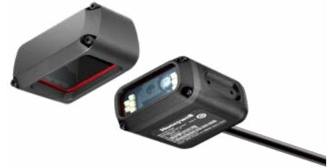
The device is integrated with network ports, RS232 port and RS485 port as well as I/O port input to meet the needs of users in different application environments. A 0-degree and 90-degree version for vertical or horizontal mounting can be selected based on the site's actual working needs.
